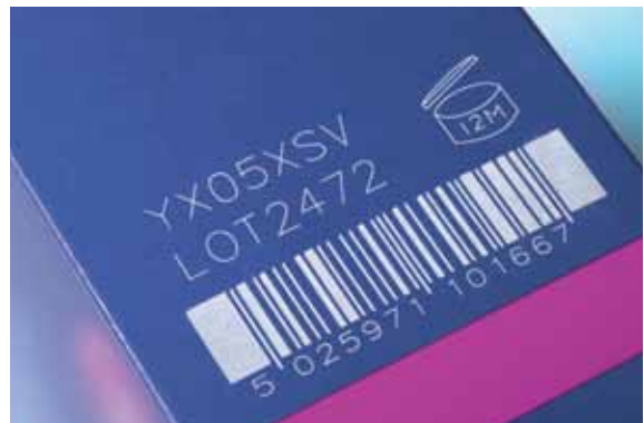
Laser printing complex code onto cosmetics packaging
