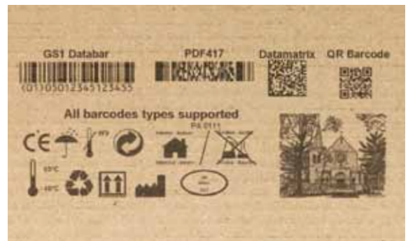
Large character printing of variable information and complex graphics onto secondary packaging
