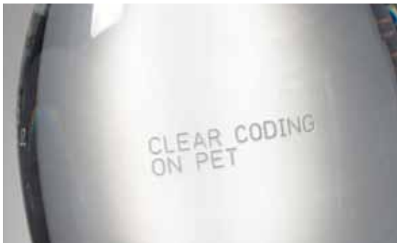
Laser coding onto PET
