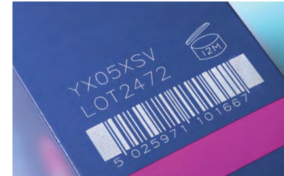
Laser printing complex code onto cosmetics packaging
