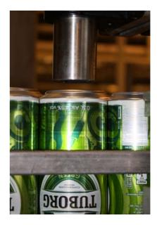
After some significant problems with its previous system the brewer purchased seven Linx continuous ink jet (CIJ) printers, which code dates on 15-20 products per second.
